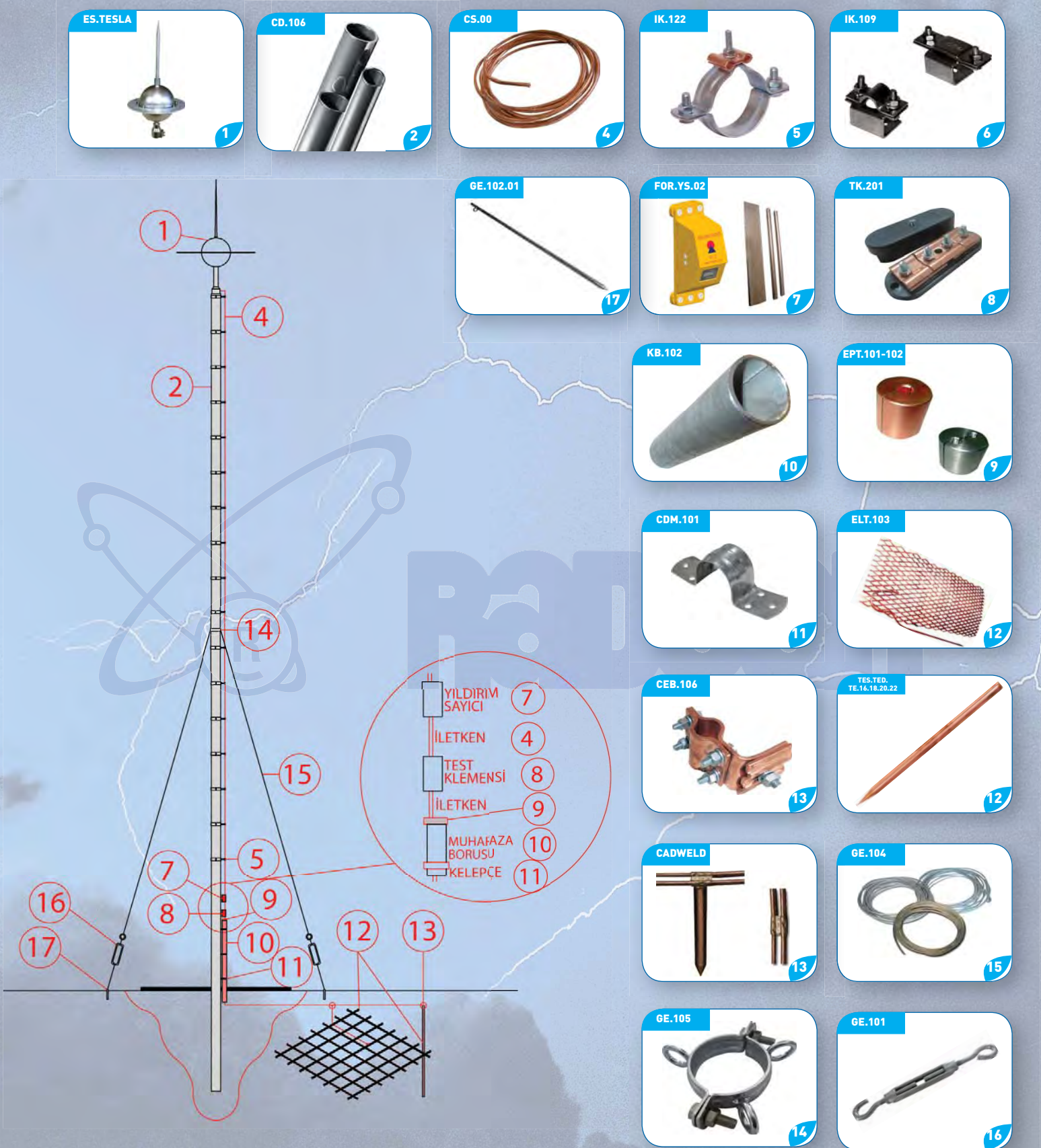
Şekil 13 Boru / Direk Paratoner ve Topraklama Uygulama Örneği Figure 13 Application example of lightning protection and grounding at a mast
